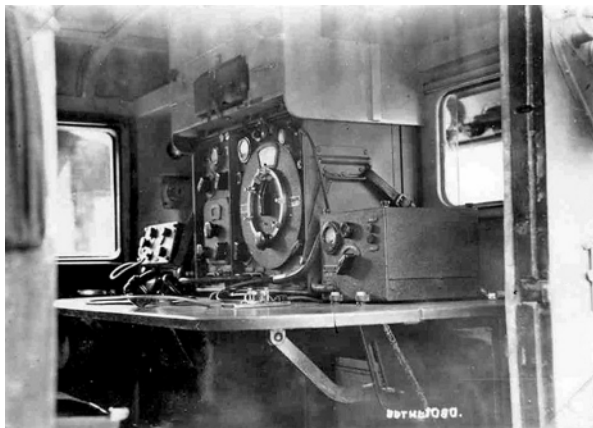
A N1/S station fitted in the rear compartment of a Polski Fiat 618 wireless version. Note the auxiliary receiver at the left and the power control/junction box at the right hand side of the transmitter-receiver.
