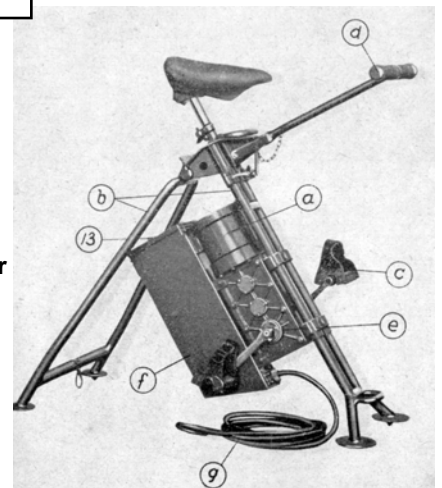
Transmitter rotary converter type RNS-39 (above).
